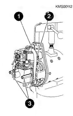
Disassembling engaging shaft
